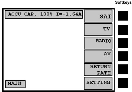
The MSK 33 is operated via a menu guided on screen representation with main menus and submenus. By means of the six softkeys, the commands displayed on the right-hand side of the TFT screen can be called up. The screen displays can be switched off for observation of the entire screen by pressing OSD/help button.
